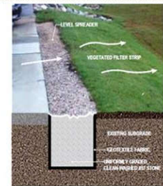
Figure VFS-1 Vegetated filter strip receiving stormwater runoff from a parking lot into a stormwater cell. Raleigh, North Carolina. Photo source: Telsa Tech, Inc. Rendering components: San Antonio River Authority.
