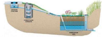
Figure TTNSB-1 Treatment Train diagram with hydrodynamic separator flowing into bioretention. Source: TerraTech, Inc.
