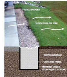
Figure VFS-1 Vegetated filter strip collecting stormwater runoff from a parking lot into a stormwater cell. Raleigh, North Carolina. Photo source: Telsa Tech, Inc. Rendering components: San Antonio River Authority.
